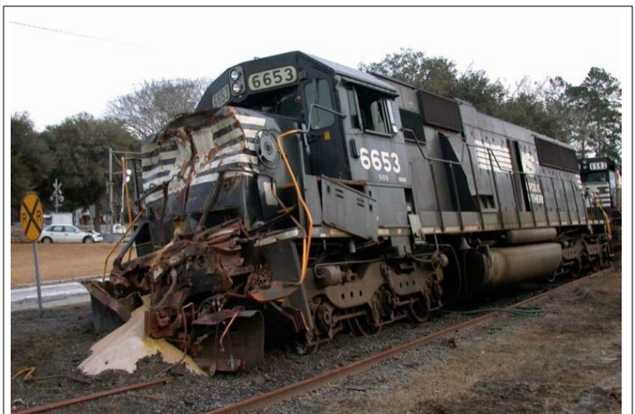
Lead locomotive in the aftermath of the NS wreck at Granite, SC in 2006 that killed nine. The NTSB recommendations for switch point indicators in dark territory went unheeded by the rail carriers and the FRA, as did a more modest proposal for restricted speed to avoid such collisions. In both cases, the railroads complained of the exorbitant expense of such installations or operations.
